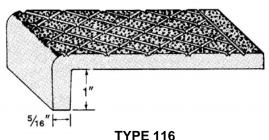
Standard nose - 1" Standard thickness - 5/16" Standard widths - 3", 4" and 6" DRAWING NOT TO SCALE
