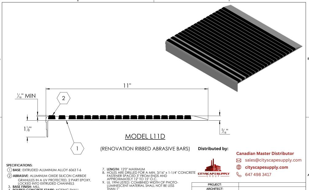
4. POURED CONCRETE STAIRS: NOSING SHALL TERMINATE NO MORE THEN 3" FROM END OF STEPS
